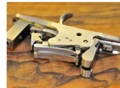
Above: A trigger plate action ready to be fitted to a superb Bosis shotgun.
